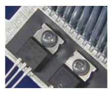
Sil-Pad 1200 is a silicone based, fiberglass-reinforced thermal interface material featuring a smooth, highly compliant surface. The material features a non-tacky surface for efficient re-positioning and ease of use, as well as an optional adhesive coating. Sil-Pad 1200 exhibits exceptional thermal performance at low and high application pressures. The material is ideal for placement between electronic power devices and a heatsink for screw and clip mounted applications.
