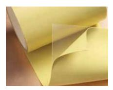
Sil-Pad 1100ST (Soft Tack) is a fiberglass-reinforced thermal interface material featuring inherent tack on both sides. The material exhibits excellent thermal performance at low mounting pressures. The material is supplied on two liners for exceptionally easy handling prior to auto-placement in high-volume assemblies. The material is ideal for placement between an electronic power device and its heat sink.
