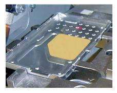
Hi-Flow 650P is a thermally conductive phase change material, reinforced with a polyimide film that is naturally tacky on one side. The polyimide film provides a high dielectric strength and high cut through resistance. Hi-Flow 650P offers high temperature reliability ideal for automotive applications.
