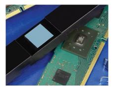
Hi-Flow 565UT is a naturally tacky, thermally conductive phase change material which is supplied in an easy to use tabulated pad form. In the application the material undergoes a phase change softening, starting near 52°C. The phase change softening feature improves handling characteristics prior to assembly. At application temperatures and pressures, Hi-Flow 565UT wets out the thermal interfaces resulting in a very low thermal impedance.
