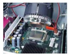
Hi-Flow 225U is designed for use as a thermal interface material between a computer processor and a heat sink. The product consists of a thermally conductive 55°C phase change compound coated on a release liner and supplied on a carrier.
