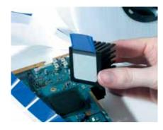
Bergquist Bond-Ply 400 is an un-reinforced, thermally conductive, pressure sensitive adhesive tape. The tape is supplied with protective topside tabs and a carrier liner. Bond-Ply 400 is designed to attain high bond strength to a variety of "low energy" surfaces, including many plastics, while maintaining high bond strength with long term exposure to heat and high humidity.
